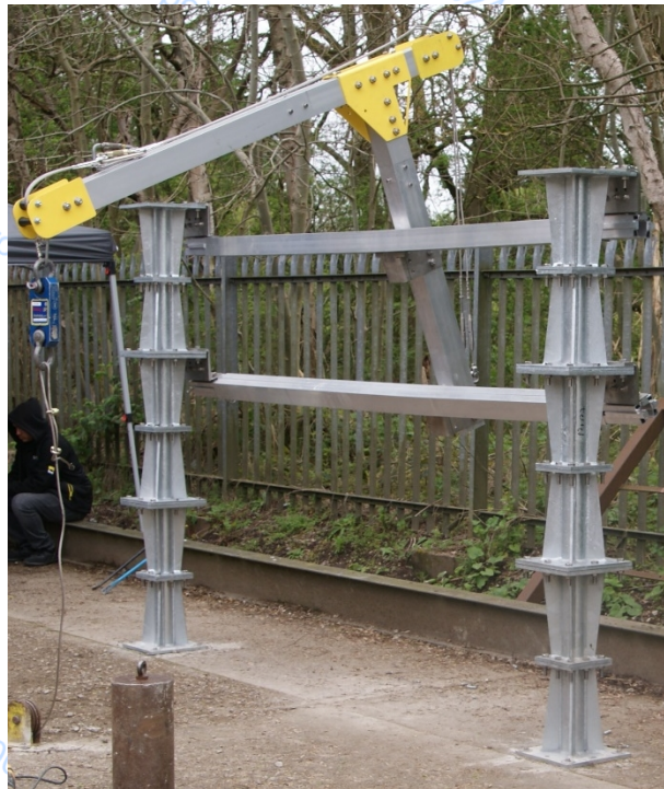
Figure 2 – Anchor rail described as “ERD.1500.1500 EdgeReil Davit” mounted on a stack of 6 davit bases
